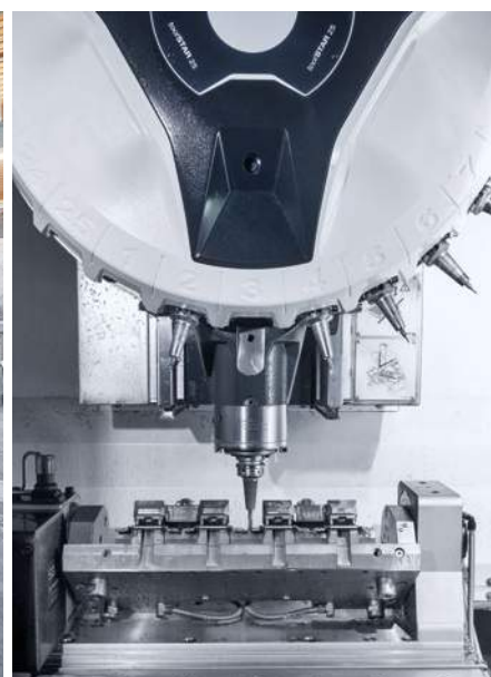
The workholding was specially designed for the process and has space for four workpieces.
