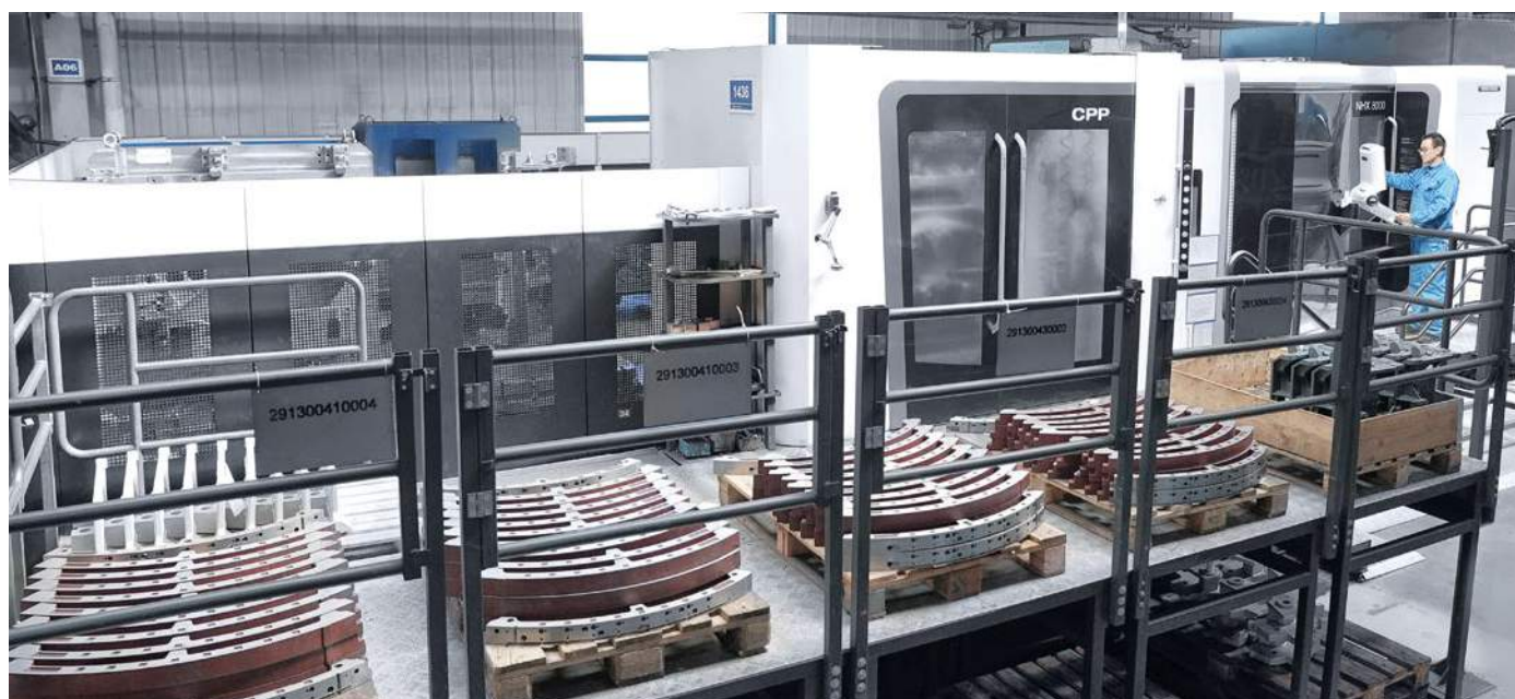
Trützschler uses an NHX with a 7-station carrier pallet pool (CPP) for automated manufacturing of large components.
