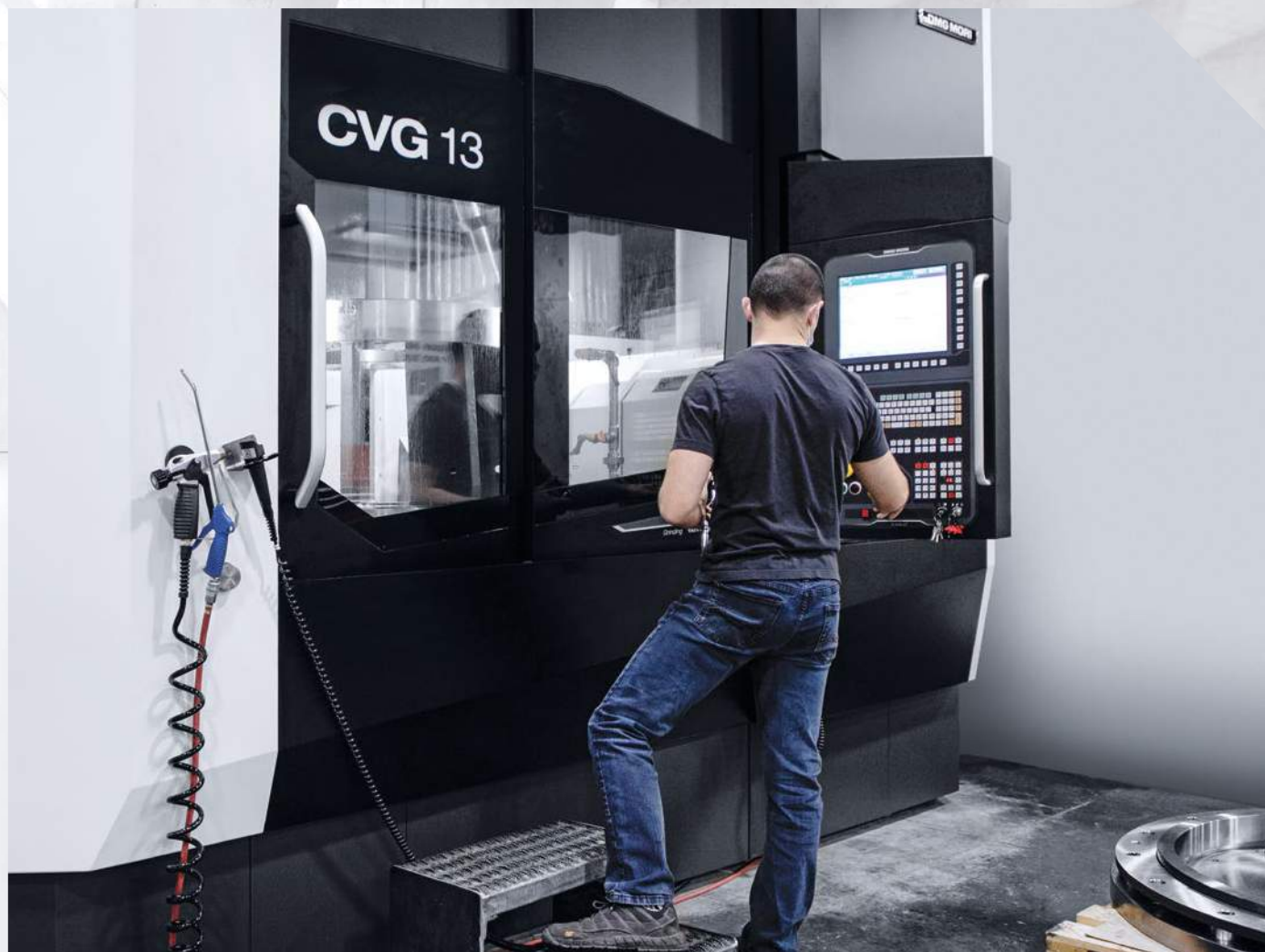
For the finishing process, NAMCO uses among other machines a CVG 13. Large components with a diameter of up to 1,300 mm are ground.
