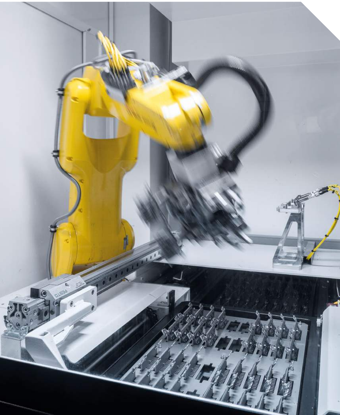
The WH 3 workpiece storage serving the DMP 70 offers space for up to 600 parts, enabling unattended production for up to 15 h.
