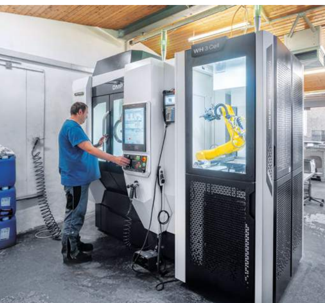
Griesshaber manufactures over 4,000 headlight components per week in 3-shift operation in a footprint of less than 9 m².
