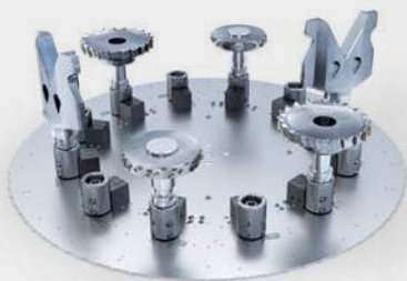
Up to 6 HSK63 tools of max. \varnothing 355 \times 370 mm and max. 30 kg weight
