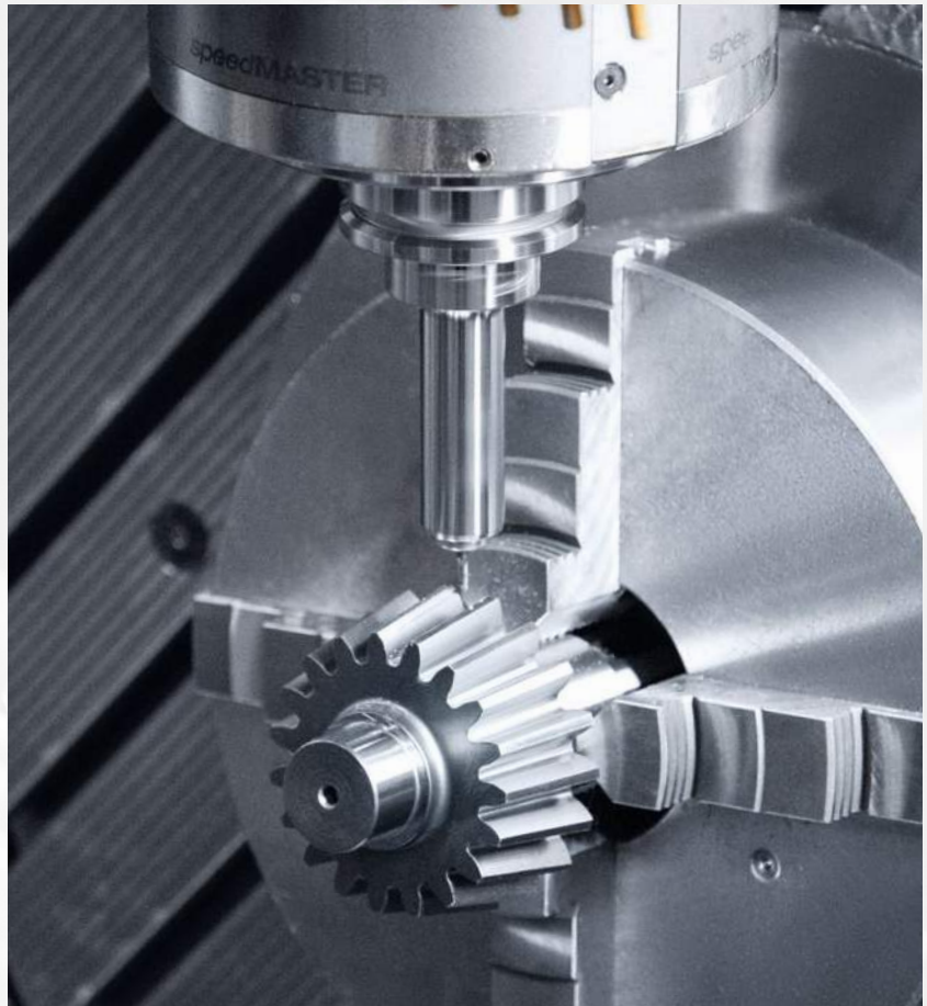
For smaller special gears, NAMCO uses, among other things, a DMU 65 monoBLOCK, which is automated with a PH 150.
