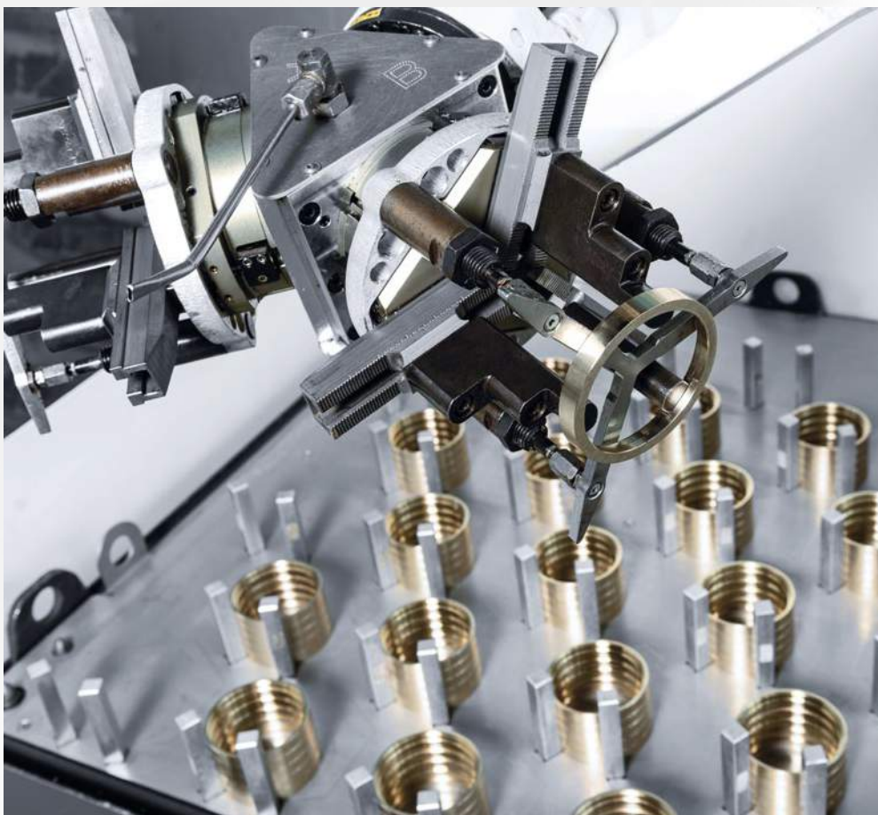
The Robo2Go stacking magazine offers sufficient capacity to enable around-the-clock production with the CTX beta 800 TC.
