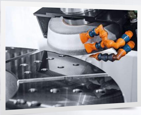
High-precision components are essential for NAMCO gearboxes. Thanks to the grinding process, surface qualities of up to Ra 0.17 µm are achieved
