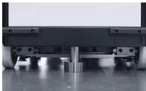
Secured via 3-point support
