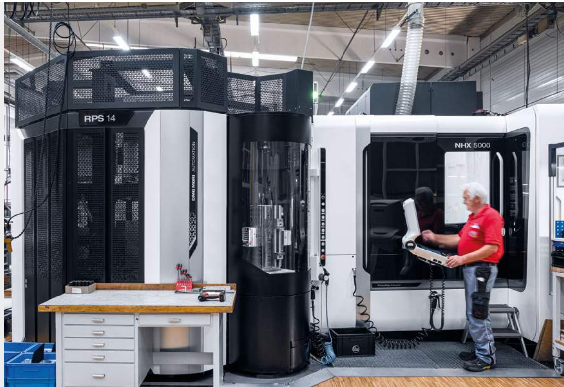
Heppler uses 3 NHX 5000s for automated manufacturing of hydraulic components made of stainless steel, which are all automated with an RPS 14-station rotary pallet storage system.
