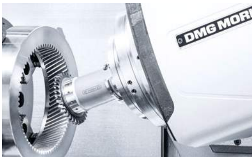
TURN & MILL Gears up to module 4 (e. g. NTX 3000 or CTX gamma TC)
