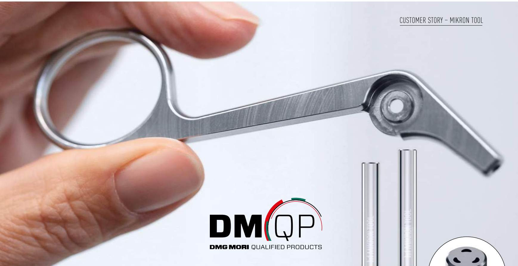
DMP 70: Machined handle of biopsy forceps made from martensitic chromium steel (1.4021/X20Cr13). The CrazyDrill SST-Inox IK is used for drilling the hole.
